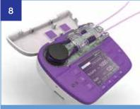
Insert the giving set into the pump and open the clamps on the 2-Pack connector
