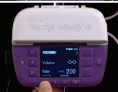
The green light on the **run** symbol indicates that the pump is working.
