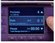
Once the portion and rate have been set, the portion run time is displayed below the rate.
