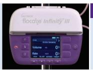
7 Then select volume and set volume by pressing the +/- buttons. Press the middle button to confirm.
