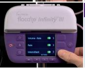
Then select **rate** and set rate by pressing the **+/**-buttons. Press the **middle** button to confirm.
